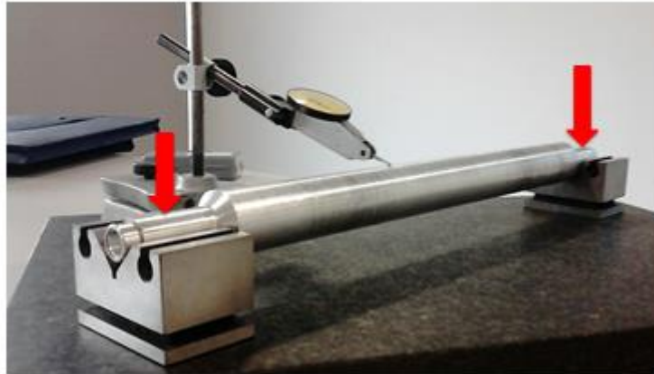
Robust Datum constructed from two faces.
