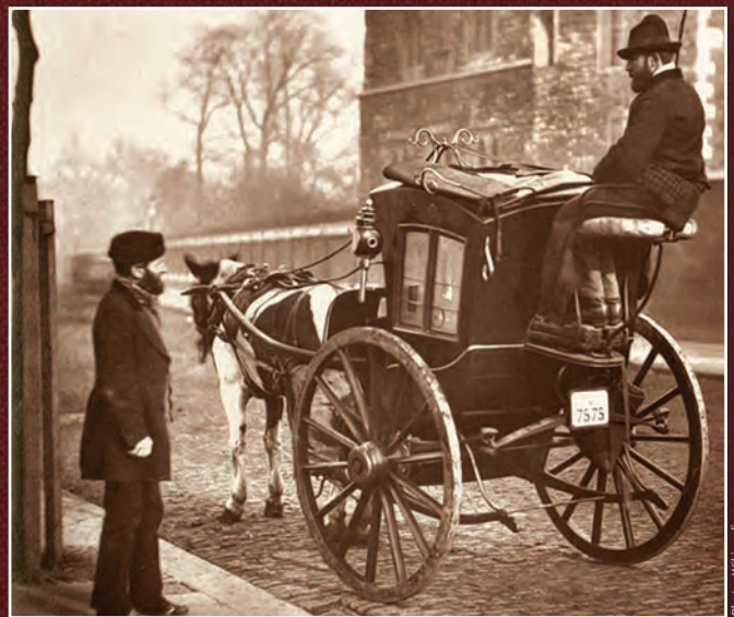
Photograph of a Hansom cab from "Street Life in London" 1877 by John Thompson and Adolphe Smith. This agile vehicle seated two passengers with the driver outside at the back of the vehicle. It was fast and easy to maneuver.
