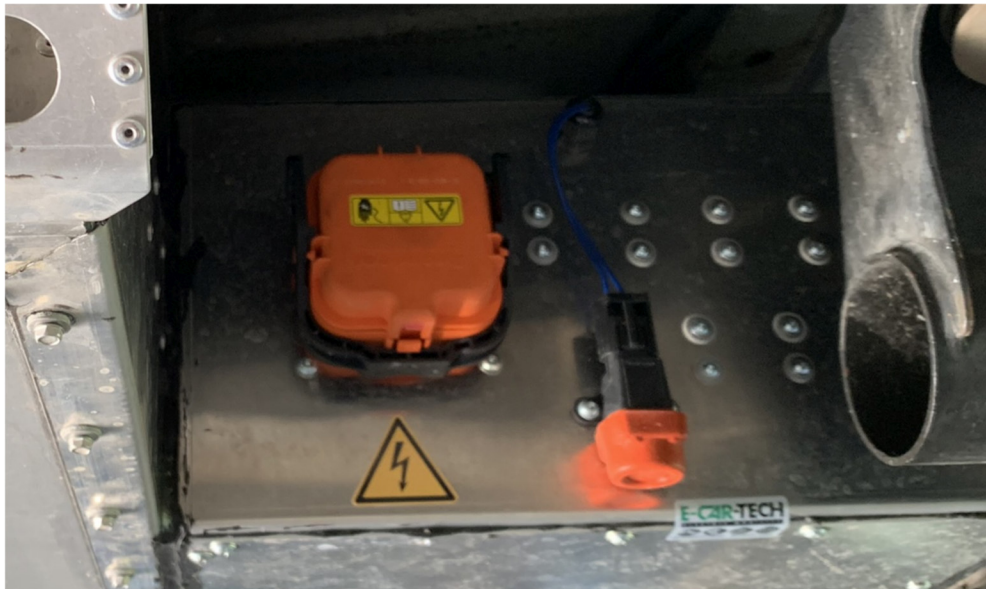
Position Service Disconnect (orange).
