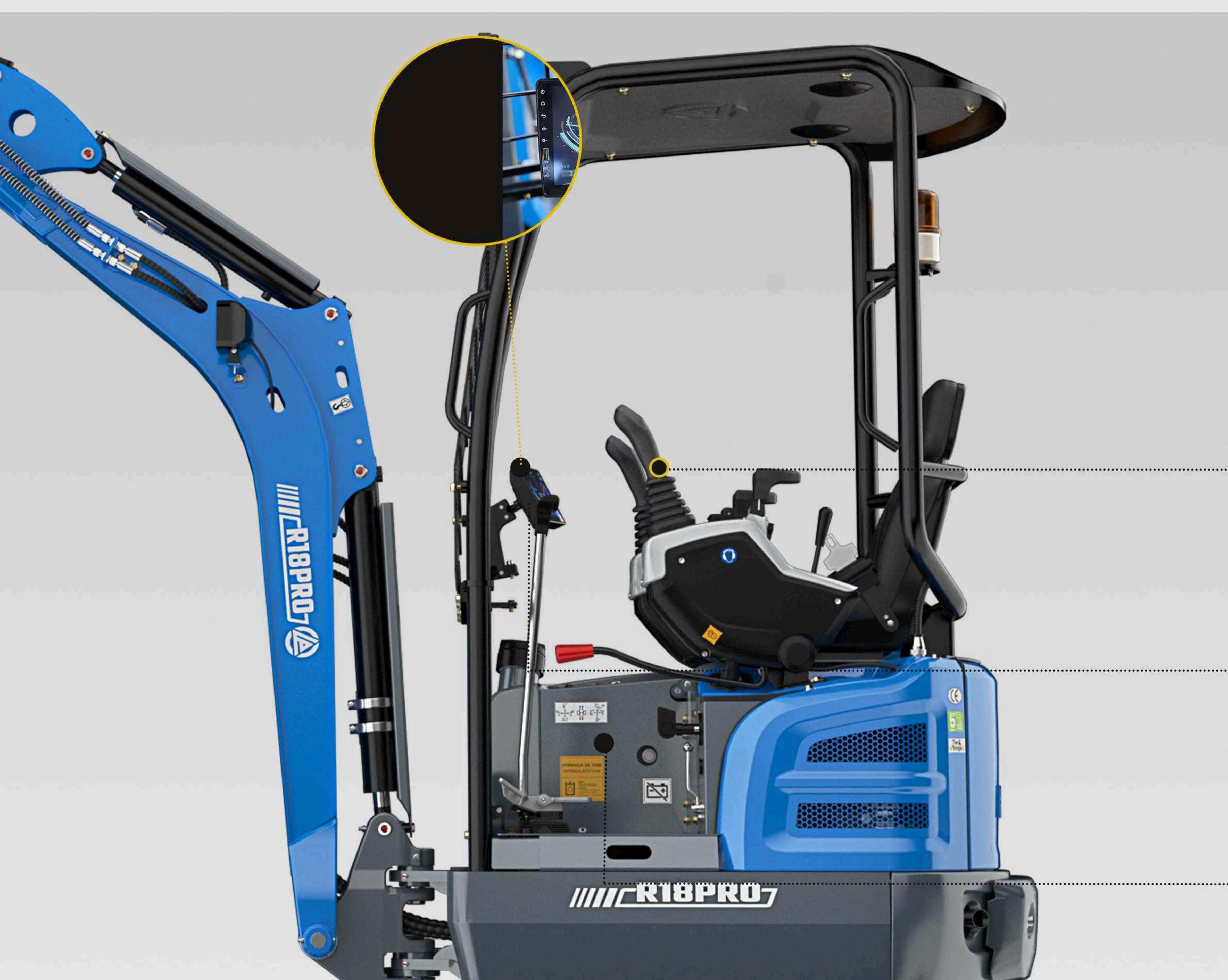
**Everything in clear sight and under control.** The modular control lever stays allow for a completely new operating concept with the greatest level of clarity and safety. Everything is within reach here and is clearly arranged through the perfect integration of the switch panel, display element, proportional control, throttle lever, adjustable arm rests and dozer blade lever.
