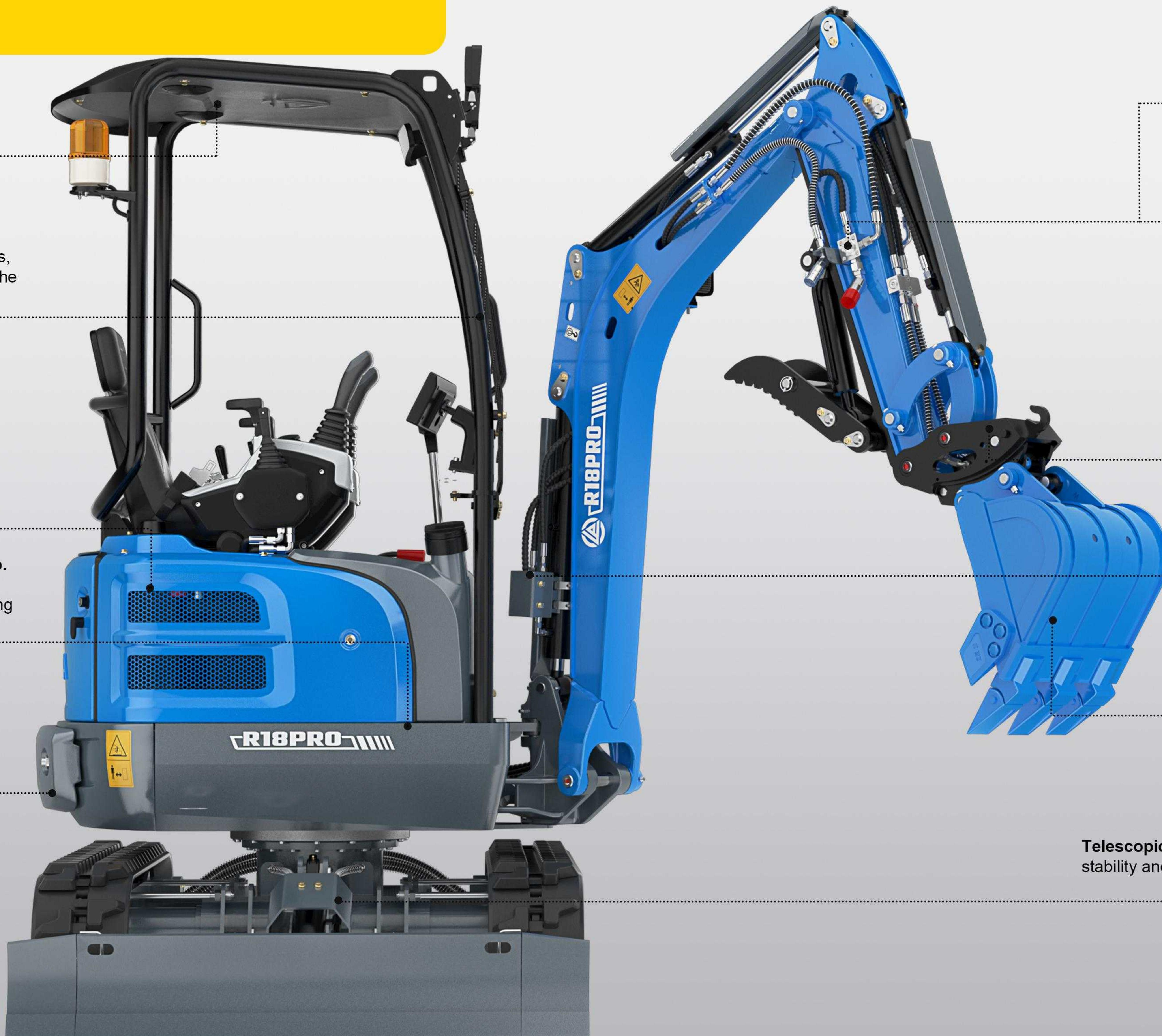
**Double action additional hydraulic unit as standard equipment.** This vastly expands the range of R18 PRO applications.
