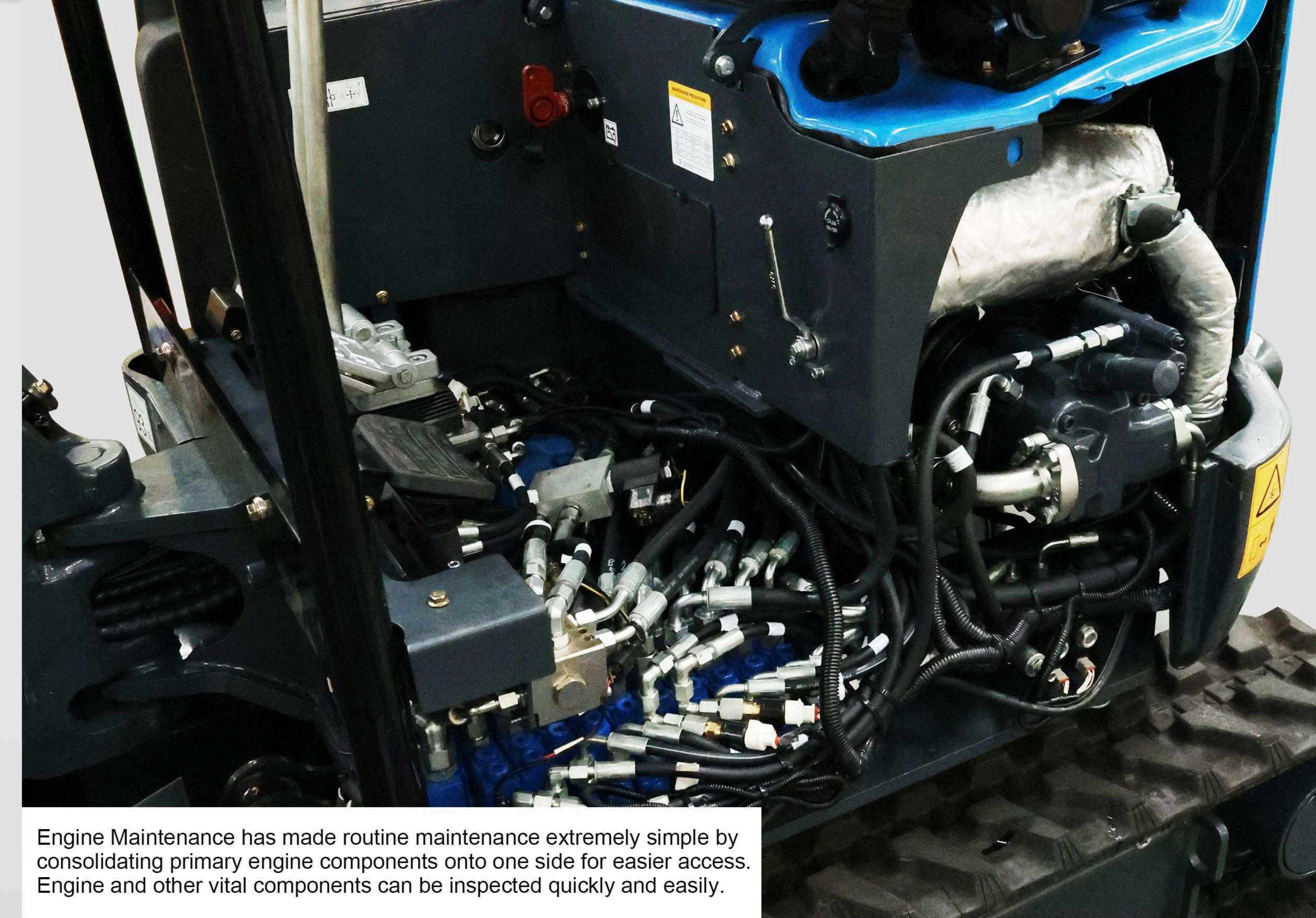
Engine Maintenance has made routine maintenance extremely simple by consolidating primary engine components onto one side for easier access. Engine and other vital components can be inspected quickly and easily.
