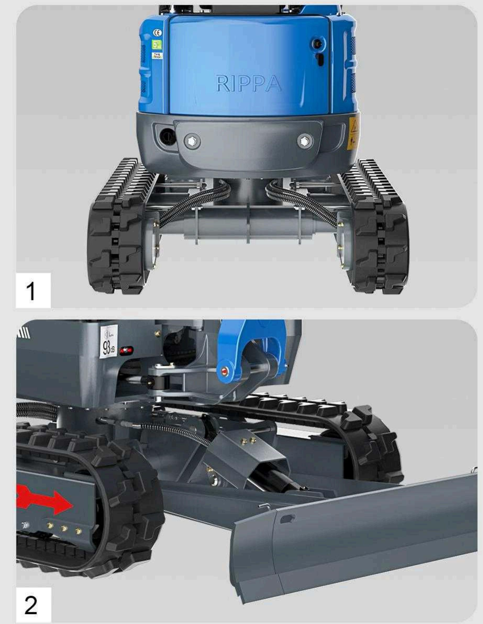
**Full safety and best protection.** The hose guide from the lifting arm to the chassis runs on the inside and is led through a two-piece pivot console. The lifting arm cylinder is positioned on the top side and therefore offers the optimal protection for the piston rod. This way, you are always at work with full safety
