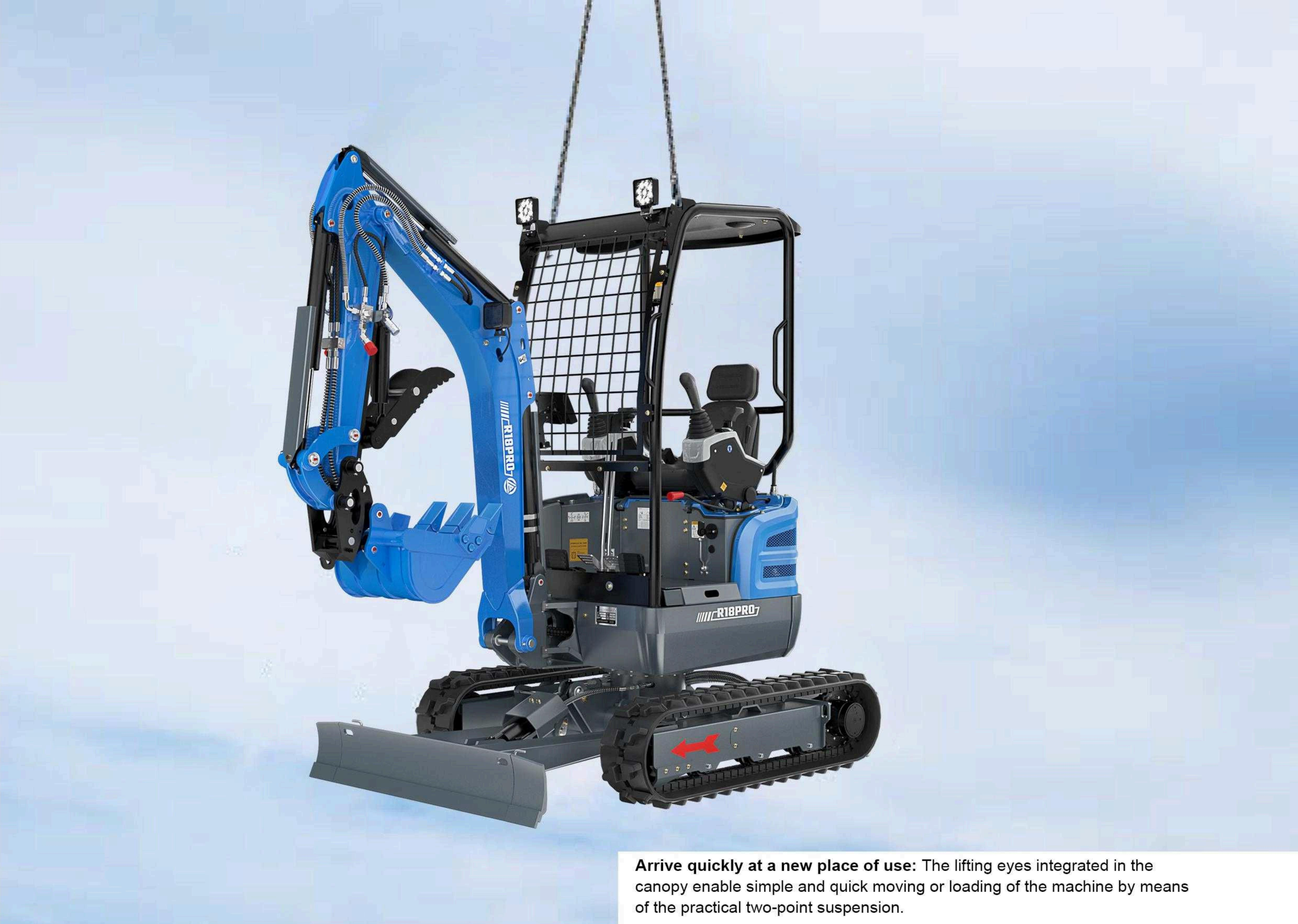
**Arrive quickly at a new place of use:** The lifting eyes integrated in the canopy enable simple and quick moving or loading of the machine by means of the practical two-point suspension.
