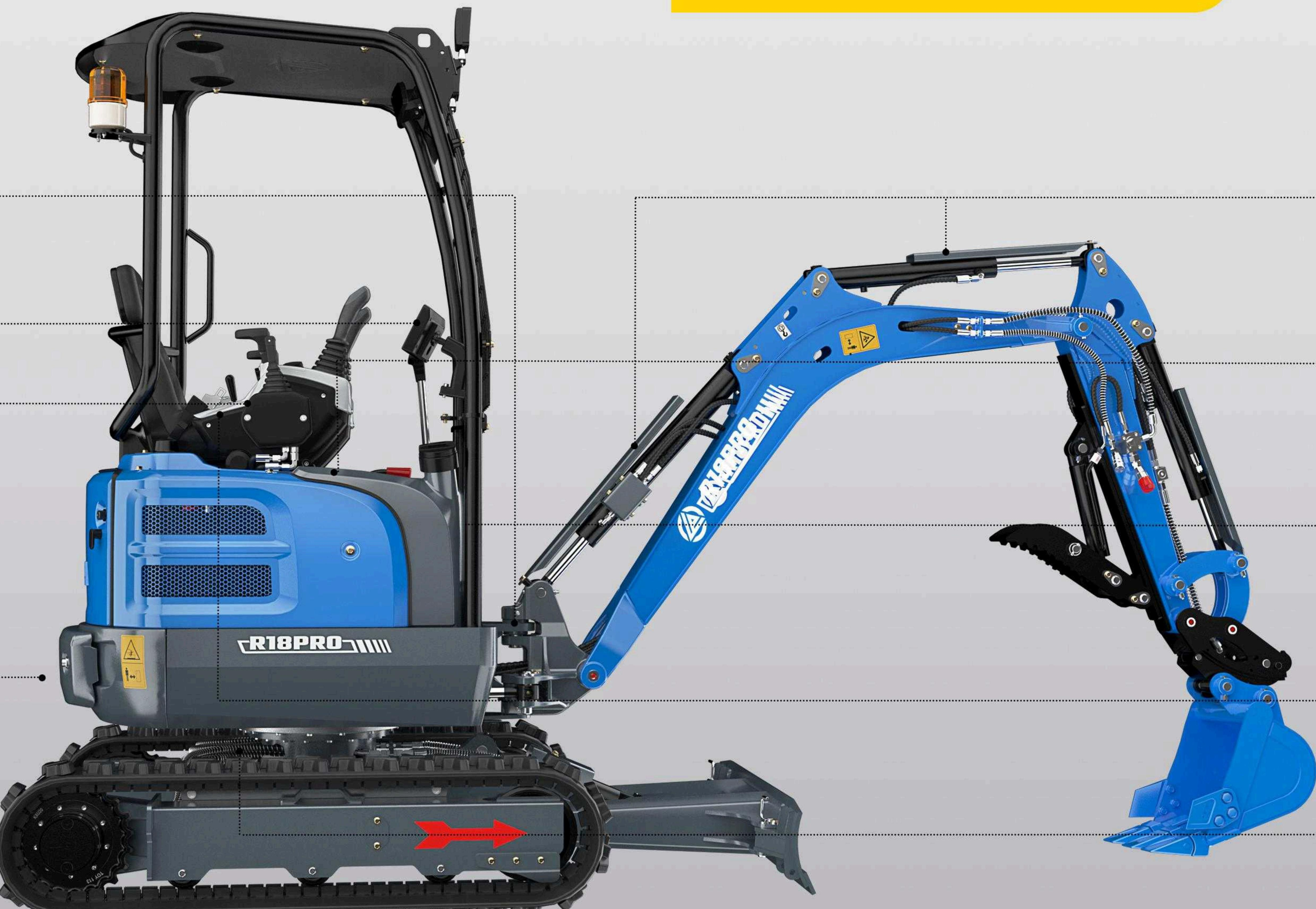
**Additional plus in safety.** A cylinder guard is added to the cylinder to effectively protect the cylinder.
