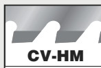
Alloyed tool steel with tungsten carbide teeth or tungsten carbide gritted cutting edge.
