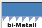
Flexible electron beam welded joint of high temperature alloyed sprung steel as backing material and high speed steel on the cutting edge to meet the highest demands given to a blade during use. Advantages against standard high speed steel blades:
