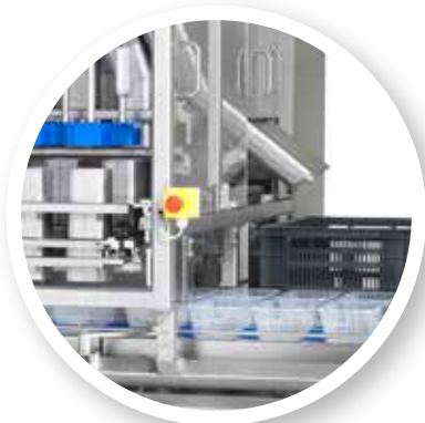
Funnel for discharge of rejected product
