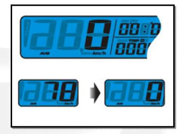
Press the **Select button** to switch from Speed Record back to main screen.
