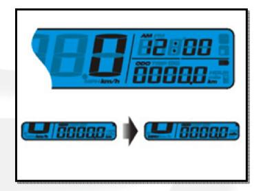
**USE OF TRIP:** In main screen, press the **Adjust button** once to switch the function from odometer to trip.
