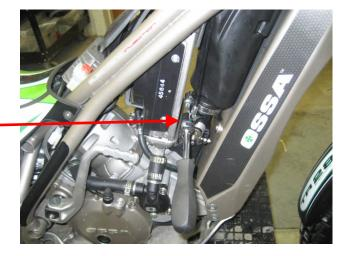
On the left side of the air box remove the temperature sensor which is press fit into the bottom of the air filter rubber,
