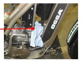
To reinstall, push clean and oiled air filter through the air box with the temperature sensor hole pointing to the left. With the throttle body out of the way you will be able to pull the air filter through from the bottom. Pull the left side through with the sensor hole first, then slide the right side through, there are pull tabs to accomplish this.
