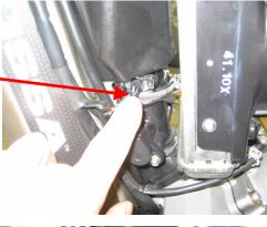
Air filter temp. sensor receiver and tabs. Tabs will be used for installation to snap sensor into position.
