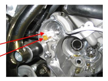
Locate the cir clip groove and rubber - stop.
