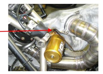
Spring adjustment is a double lock nut, can be adjusted using a drift or removing the exhaust will give full access for using the appropriate tool.
