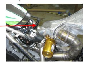
Removing the spark plug will allow a 3mm allen wrench to reach the rebound damping adjustment, increase and decrease by clicks
