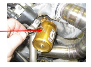
The top adjustment is for compression damping and is adjusted by clicks.
