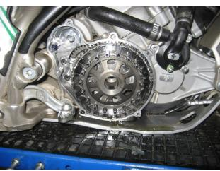
Remove 5 transmission screws using a flex 3mm hex. You will probably have to drift each screw to release the blue lock tight. You will have to rotate the the clutch gear to access the three inner screws. Take note of the half moon cut out on the clutch inner casing to allow the screws to be pulled from the transmission.
