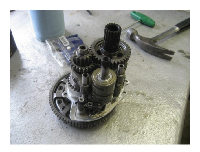
To install, as you slide the transmission in make sure the clutch gear lines up with the crank gear in this area. Just rock it back and forth to fit the gears. Don't force it.
