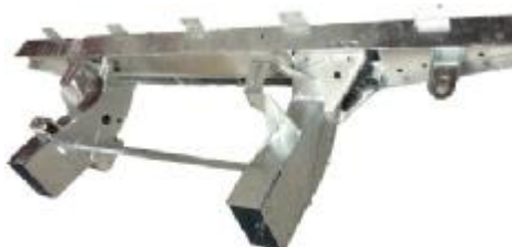
Defender 90 up to WA159806 (early type, No rear tank No rear anti roll bar) With 500mm extensions
