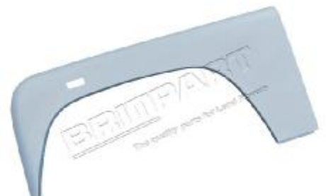
Front Wing Outer panel LH with late side repeater cut ASB710270R
