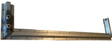
Door Frame Lower Repair Section
