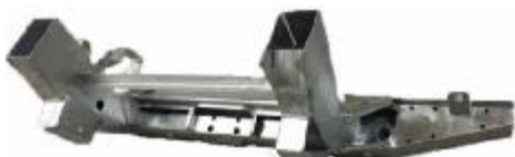
Defender 90 up to WA159806 (Early type No rear tank, with anti-roll bar mounts) With 500mm Extensions
