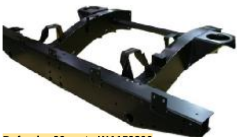
Defender 90 up to WA159806 (early type, No rear tank, No rear anti roll bar) With 900mm extensions
