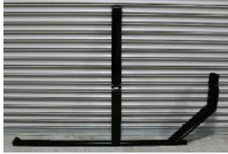
Side Frames late type for push button door handles
