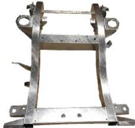
Rear Crossmember with 1400mm Chassis Legs & Fuel Tank Crossmember LRD213 Black LRD213G Galvanised
