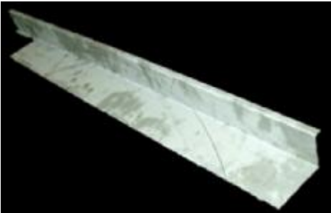
Repair Panel Bottom of Front Side Doors
