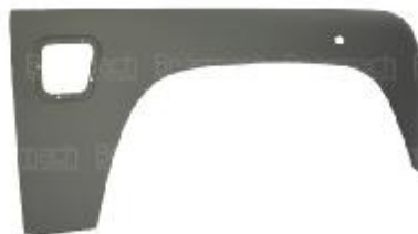
Front Wing Outer panel RH with early side repeater cut out & air intake ALR6122R
