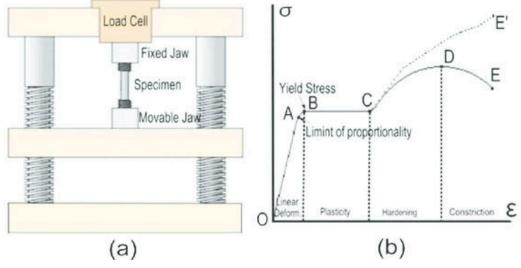
The picture above shows a strain testing machine (a) where a specimen can be exposed to a defined strain  $\epsilon$ , and the stress (force)  $\sigma$  in the material is measured. The stress-strain diagram on the right (b) shows an example of how the stress  $\sigma$  changes for a given  $\epsilon$  for a material like a construction steel. For small  $\epsilon$  values the relationship between stress and strain is linear, i.e. it can be expressed as  $\sigma$ = $\epsilon$ .
