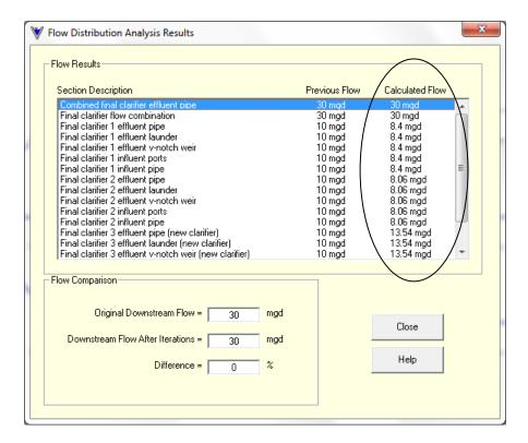
As can be seen from the results above, the path through final clarifier no. 1 receives 8.4 MGD, the path through final clarifier no. 2 receives 8.06 MGD, and the path through final clarifier no. 3 receives 13.54 MGD. Based on the elevations of the preliminary hydraulic profile, it is not surprising that the path through final clarifier no. 3 receives significantly more flow than the other 2 paths. The hydraulic profile is also updated accordingly:
