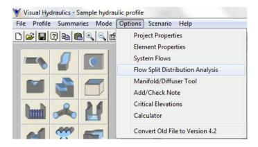
Selecting this option from the menu will instruct the software to perform a flow distribution analysis on the current hydraulic profile. The following confirmation message will be provided before proceeding:
