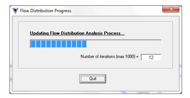
The progress screen provides the number of iterations performed as well as a progress bar that summarizes how many of the flow paths have been calibrated successfully. When all of the flow splits have been calibrated, the analysis is complete and the results will be displayed in tabular format. This summary form is shown as follows for the simple flow split just analyzed:
