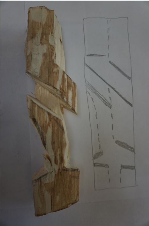
Abb. 5: Grob behauener Rohling (links) und Herstellungsschema (rechts). – Roughly hewn blank (left) and manufacturing scheme (right).
