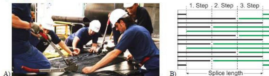
Figure 1-2: A) Preparation process of a steel cord splice [RI-Belt Sud S.R.L.]; B) Layout of a 3-step steel cord splice
