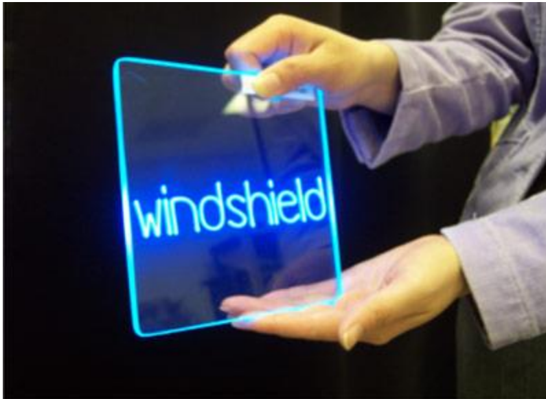
Abbildung 5-3: Emissive Projection Display (Quelle: Sun Innovations)
