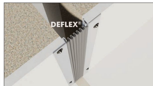
Cover profile for facades, walls and ceilings for extremely wide joints with great movement and additional cellular rubber lamination to compensate for tolerances in the substrate.
