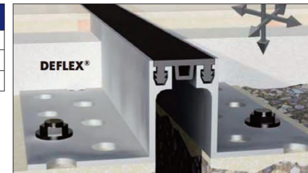
Expansion joint profile for all finishes (screed, natural stone, cast stone etc). Interchangeable insert. Smooth Insert option available (reduced flexibility). Antistatic quality possible.
