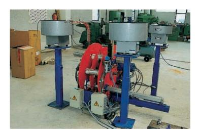
IIn four working steps: from the material feed, via precision positioning of the plastic side covers, the folding and tucking-in of the gauze sleeves, to the fixing of individual parts. The paint rollers are produced fully automatically at a rate of 650 / hour.
