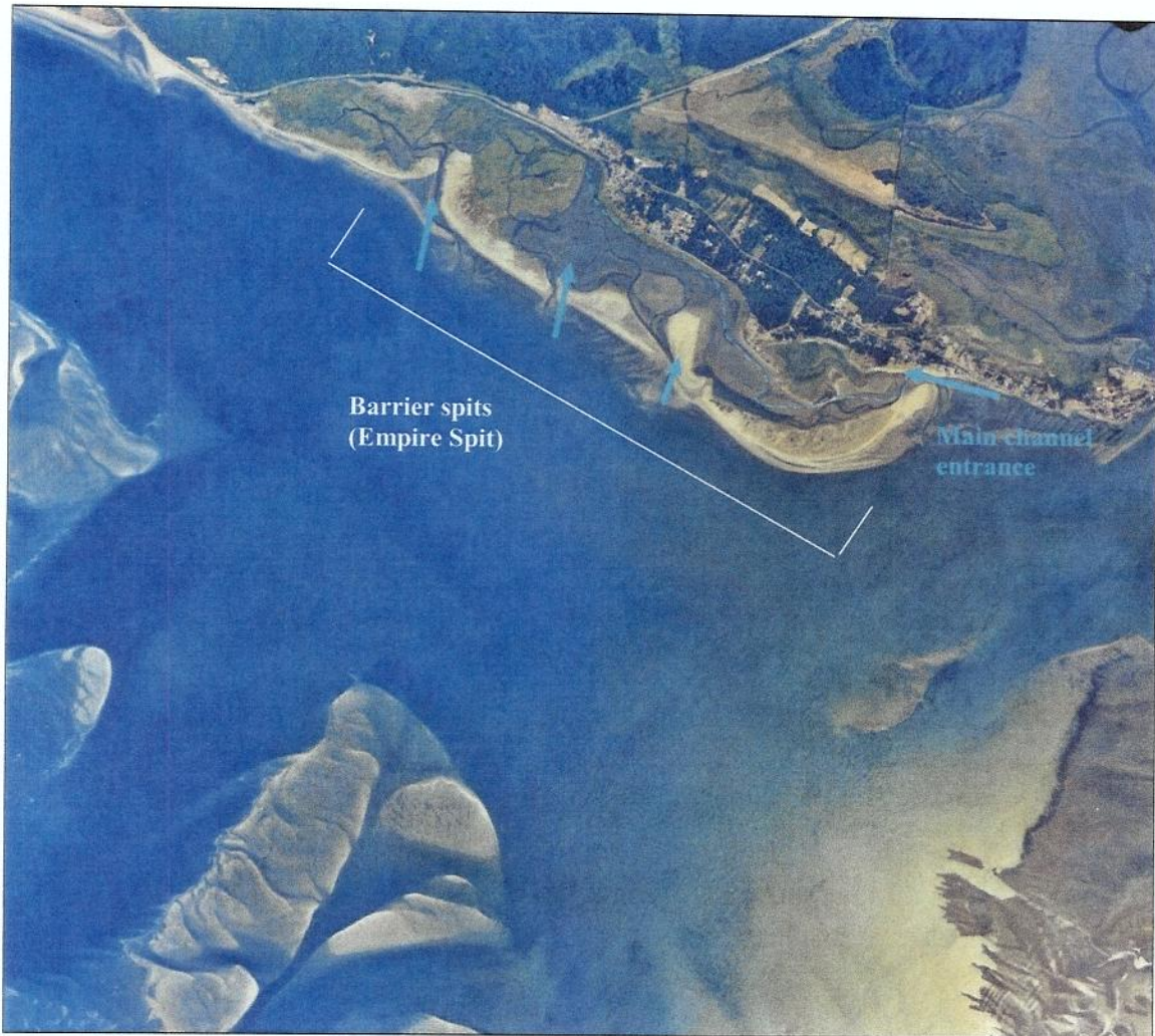
Figure 2. Barrier spits extending southeast from Cape Shoalwater (not shown), in Willapa Bay, Pacific County, Washington. (Photo courtesy U.S. Army Corps of Engineers). Arrows indicate channels into North Cove. The main channel (dotted line) now occupies areas that appear to have once been extensive tidal flats.
