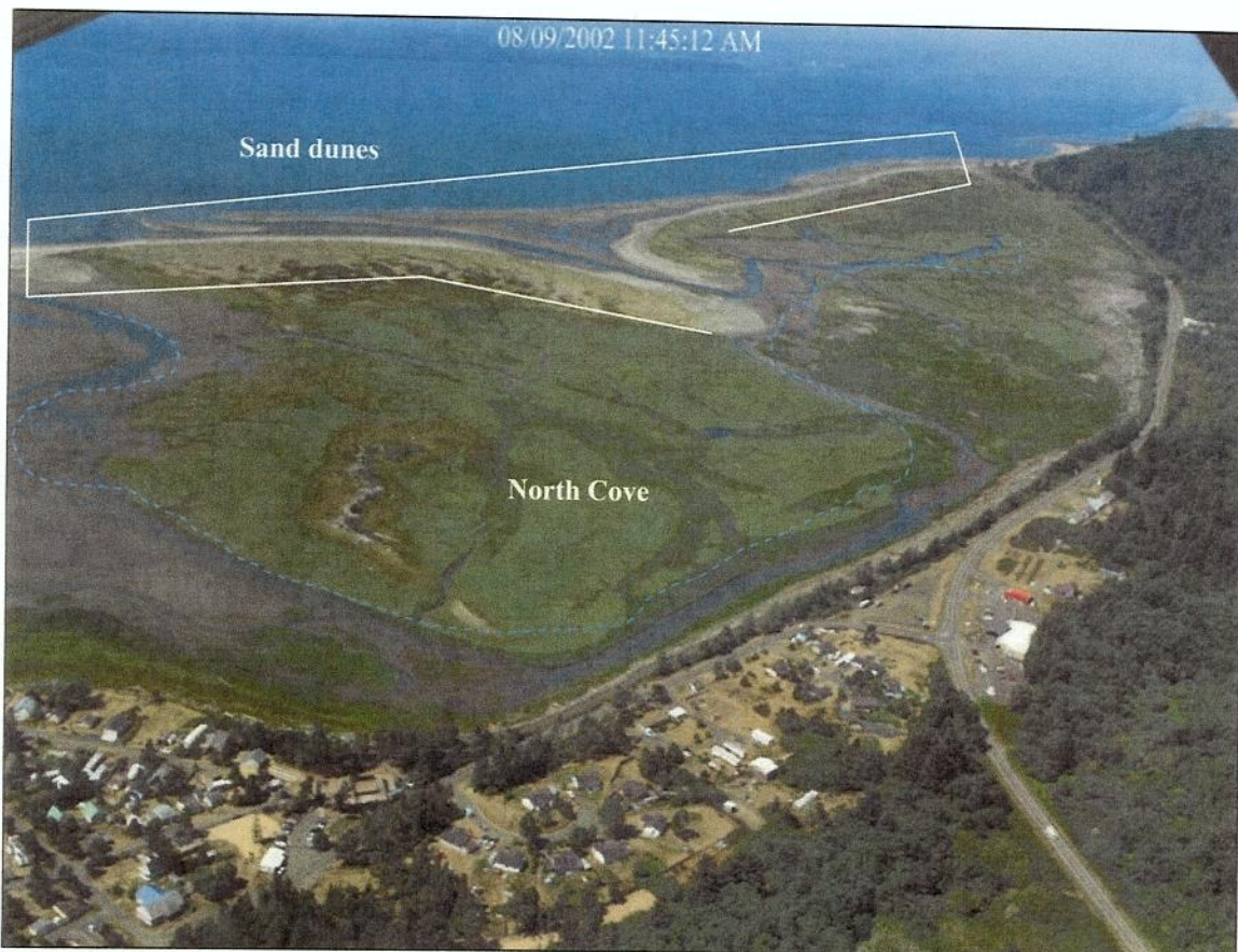
Figure 3. View of Willapa Bay and North Cove, showing location of protective sand dunes (Empire Spit). (Aerial photo courtesy of Washington State Department of Ecology). Dotted line indicates main channel. Note main breach in the protective dune.
