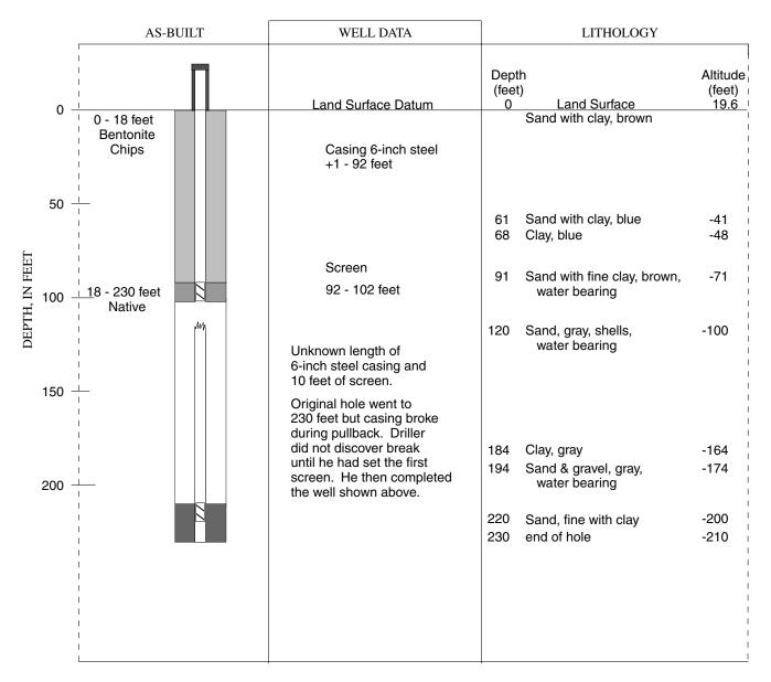
**Figure 3.** Construction, completion and generalized lithologic data for newly constructed tribal wells 14N/11W-02C01, 14N/11W-02C02, and 14N/11W-03F01.
