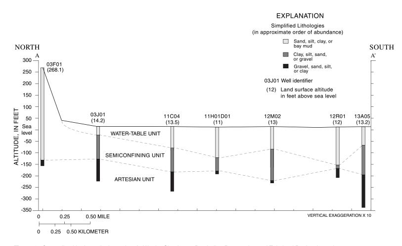
**Figure 4.** Generalized hydrogeologic section *A*-*A*' in the Shoalwater Bay Indian Reservation and Tokeland Peninsula study area. Trace of the section is shown on figure 1. See table 3 for detailed lithologies of wells.
