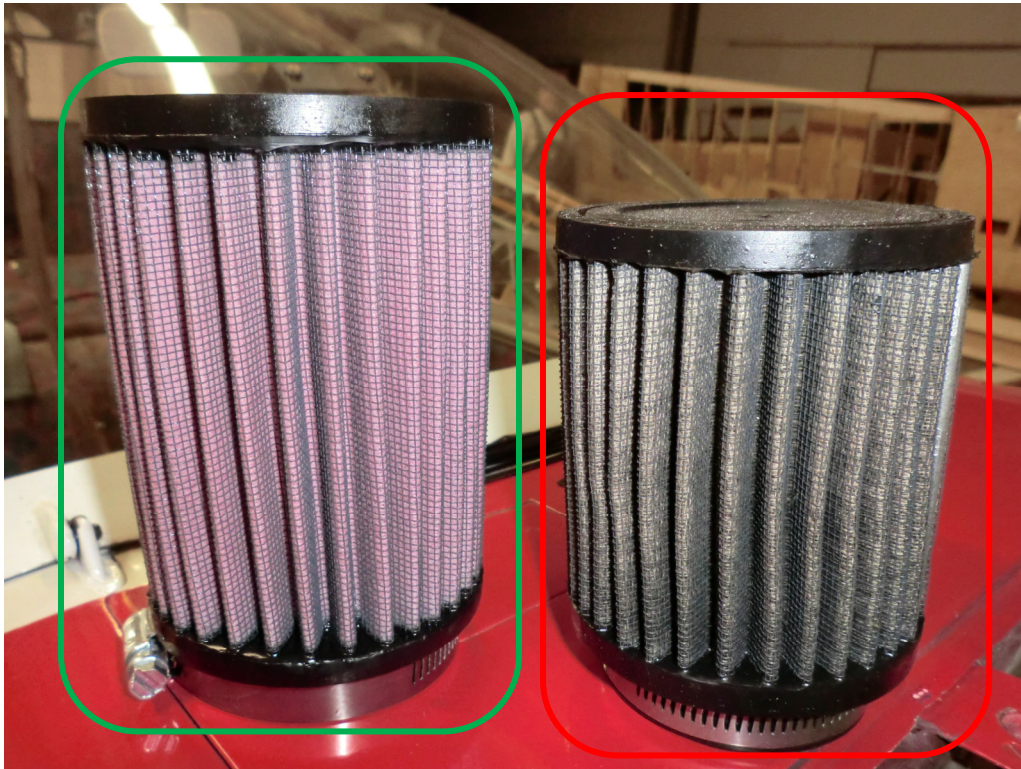
Originalluftfilter links, rechter Luftfilter zu klein / Original air filter left, right air filter too small
