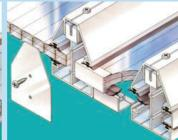
Conforming to BS 5516 the system has been designed for both the commercial and domestic markets and can be used with all popular fills including 6mm glass, multi-wall polycarbonate sheet and double glazed units. The gaskets are designed to ensure the fills are sealed even when glazed at an angle.
