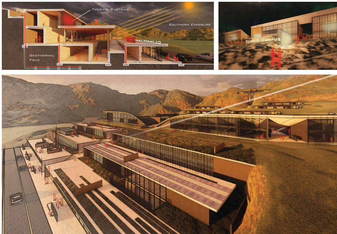
Figure 6. Embedded Community Thermal flows and wayfinding strategies, by Daniel Cusmano and Cameron Germond.
