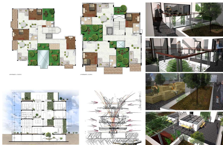
Figure 6: A building block is transformed into a multi-dwelling unit based on the vernacular courtyard typology, Larnaca, Cyprus. UNIC Student name: Maria Georgiou, Sophie Savvidou. Supervisor Anna Efstathiou.
