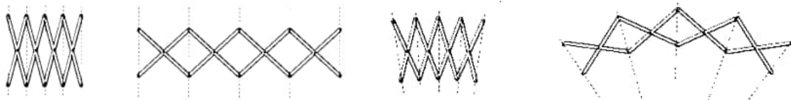
Figure 2. A deployable structure composed of multiple r-SLE units: translational unit (left) and polar unit (right) [10]
