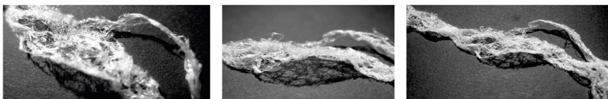
Figure 4. Application Method One - 3D printing bioplastic using a candy floss machine
