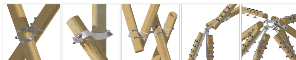
Figure 9. Connections (from left to right): 2-bar pin connection, translatable pin connection, 4-bar pin connection with screw, 4-bars pin connection with plate (for linear arrangement), and 4-bars pin connection with plate (for centralized arrangement)
