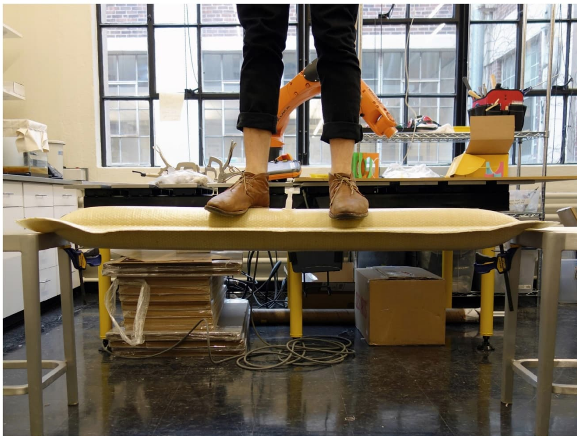
Figure 6. Costanza, David; Fibrous Tectonics Material Research, Inflatable Mold with Bio-Resin Infused Burlap, 2015.
