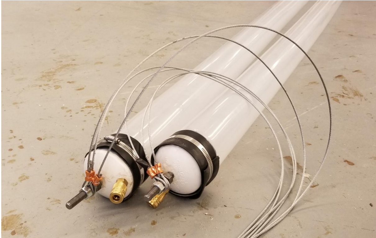
Figure 6. End-cap and valve detail with tension cables. Shown with 2 layers of HDPE tubing.
