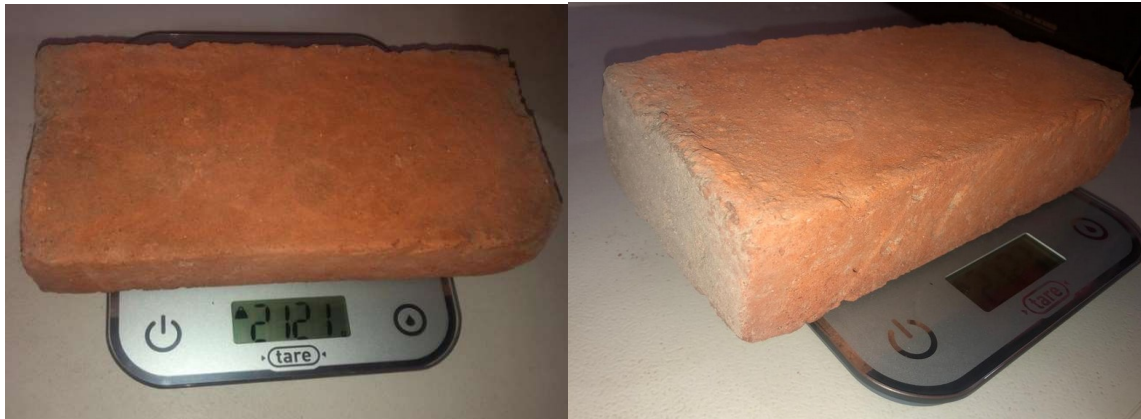
Figure 1. Weight in kg of a red brick manufactured in San Luis Huexotla, Texcoco, State of Mexico, Mexico.
