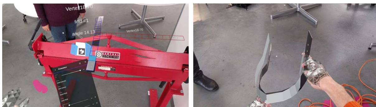
Figure 03. Steel metal fabrication with Augmented Reality
