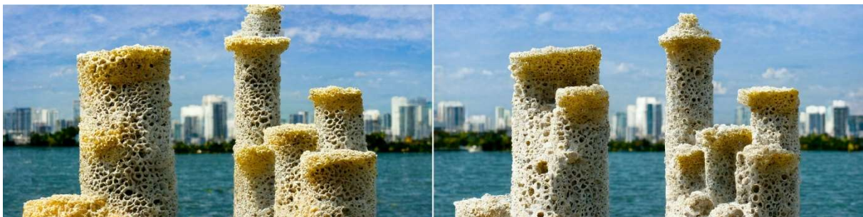
Figure 2. Render of self-growing bio-concrete structures using re-engineered cyanobacteria that deposit calcium carbonate on the crest of the structure as it rises, Biscayne Bay, FL.
