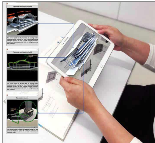
Figure 5. Animation showing the roof structure under lateral loading for Kansai International Airport designed by Renzo Piano
