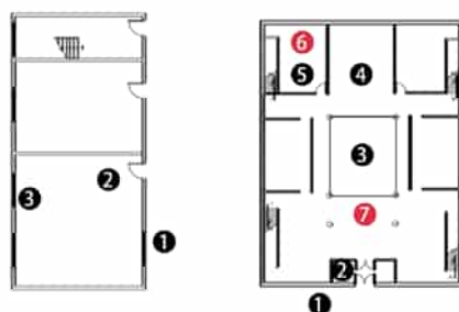
Figure 8. measurement points in modern dwelling and traditional dwelling
