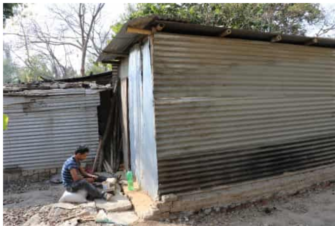
Figure 3: Self-built temporary shelter using metal sheeting in Nepal, Photo credit: D.Albadra
