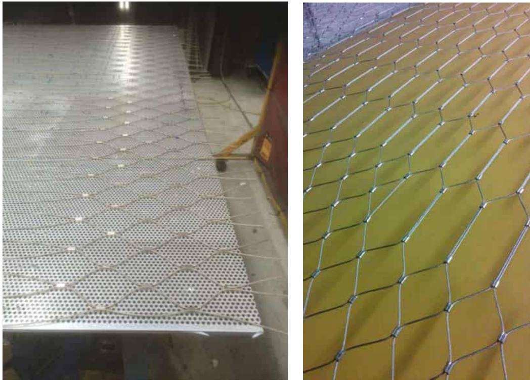
Figure 11: Photograph (LHS) showing weaving on perforated sheet, and photograph (RHS) showing tensioned wire set in frame ready for installation.
