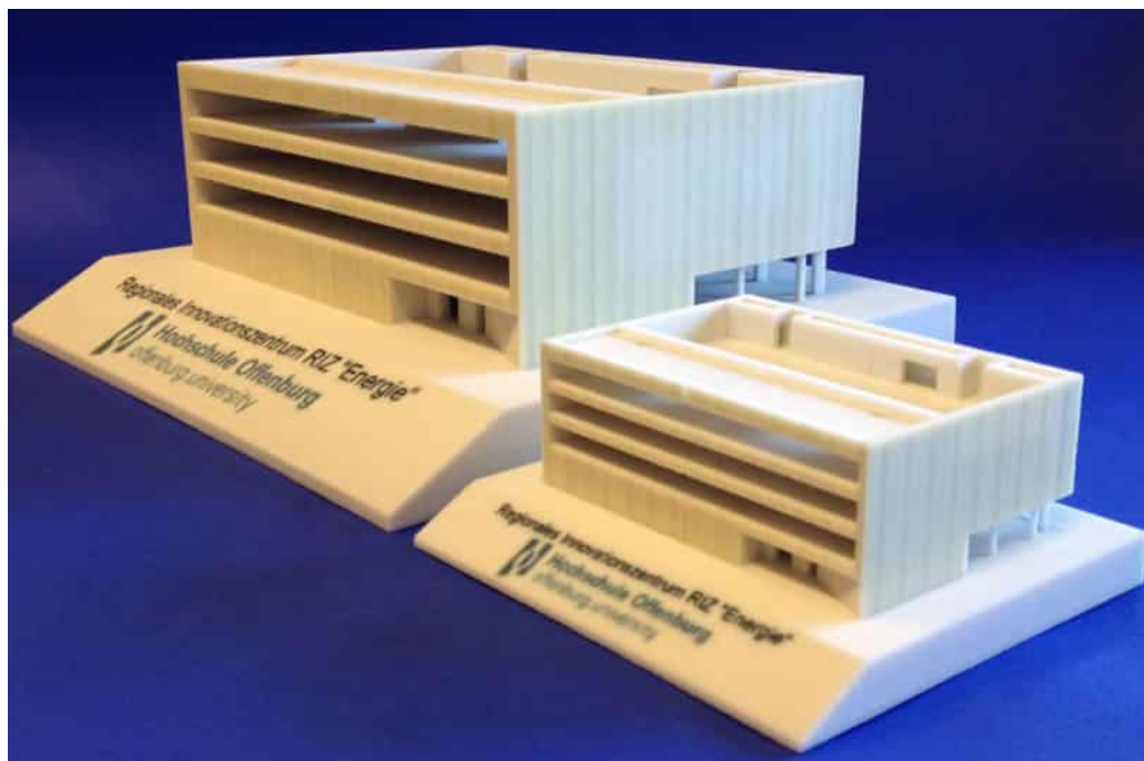
Figure 6. Parametrized architectural model in scale 1:250 (left) and scale 1:500 (right) manufactured by Binder Jetting
