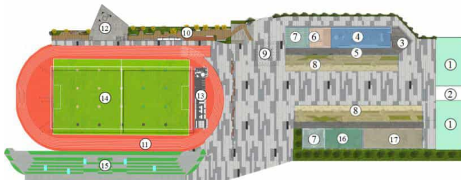
1.building A 2. school main entrane 3.indoor exhibition entrance 4.exhibition hall 5.drone/UAV display 6.office 7.WCs 8.outdoor green 9.interactive sound fountain 10.transitional area 11.existing sport track 12.observation tower 13.entrance of drone/UAV field 14.drone/UAV field 15.audiance area 16. Drone/UAV sales 17.coffee/dining
