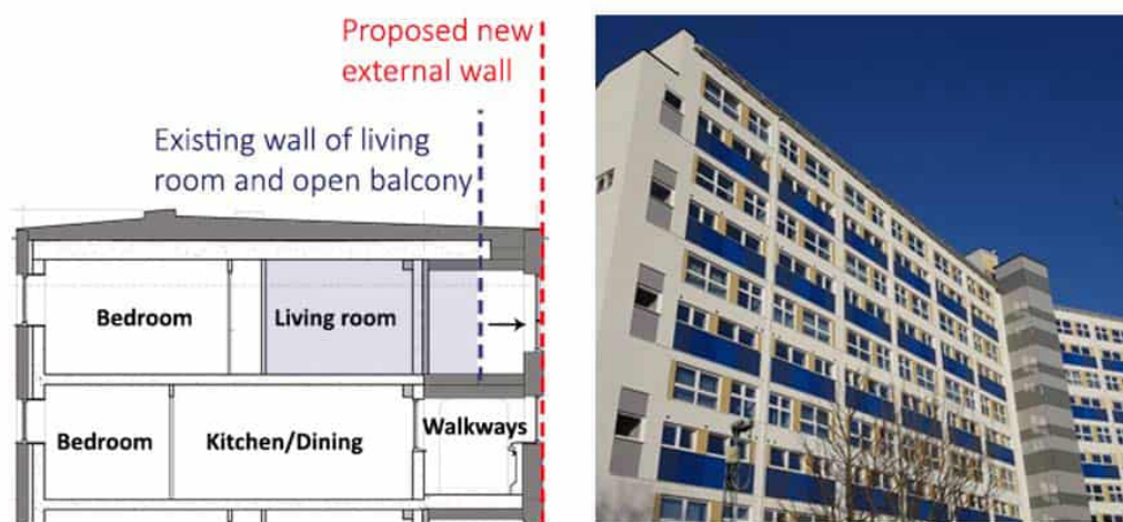
Figure 2. The design of the rear façade of Wilmcote House
