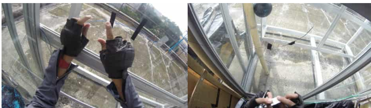
Figure 4. (Left) Putting sensor on inner side of outer skin T81. (Right) Putting sensor on inner side of first skin on model DSF.
