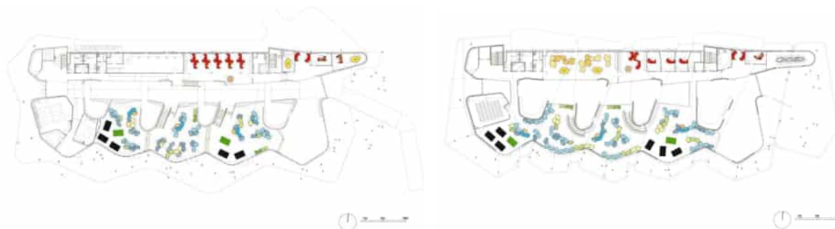
Figure 5. Final floor plans of the Abedian School of Architecture; (left) the ground floor that follows the contours of the site from the eastern entry to the higher ground in the west, and (right) the mezzanine floor, both with the two-story-high ‘Forum’ on the lower right hand corner ( https://www.archdaily.com/465030/abedian-school-of-architecture-crab-studio ).
