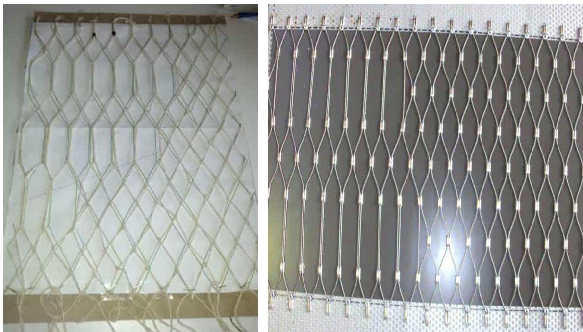
Figure 9: Photograph (LHS) showing initial 1:2 woven string prototype to test documentation method, and photograph (RHS) showing first full scale wire sample test.
