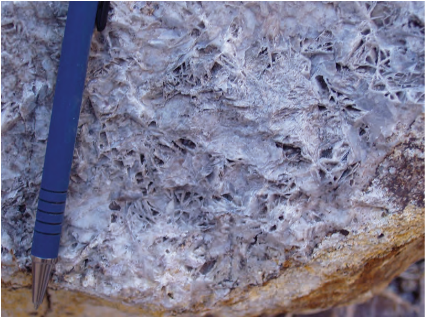
Figure 3. Angel wing texture in quartz (QW) is an “index fossil” for gold in epithermal deposits. The acute angles assumed by the quartz are reported to be after pre-existing carbonate that precipitated because of boiling.
