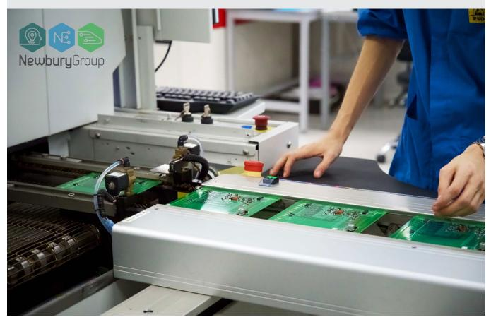
"We chose the Heller reflow ovens due to their reduced energy consumption and ability to reflow large BGA devices with a high thermal mass."
