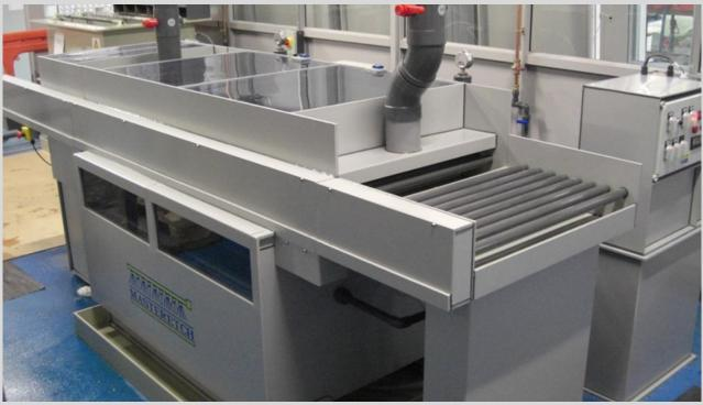
Conveyor width 750mm (30") Conveyor control DC shunt motor with digital readout speed control Conveyor drive 1 to 1 polypropylene drive gears 2.2kw glandless submersible unit Pump Filter external access lift out filter baskets Heating 3kw titanium element Temperature control Digital readout electronic thermostat Spray banks 6 top 6 bottom, quick release fan jets Carryover gap 4 sets squeegee rollers to prevent solution carryover
