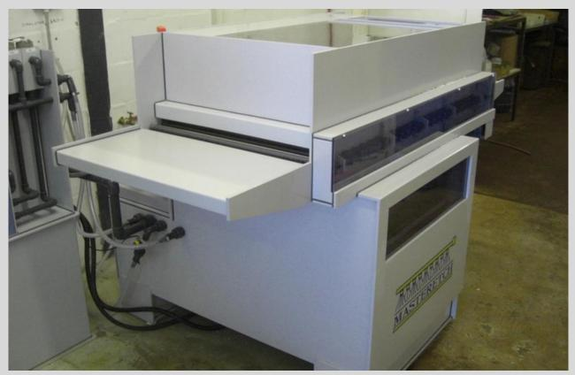
Conveyor width 750mm (30") DC shunt motor with digital readout speed control Conveyor control Conveyor drive 1 to 1 polypropylene drive gears Pump 2.2kw glandless submersible unit Filter external access lift out filter baskets Heating 3kw titanium element Temperature control Digital readout electronic thermostat Spray banks 6 top 6 bottom, quick release fan jets Carryover gap 4 sets squeegee rollers to prevent solution carryover
