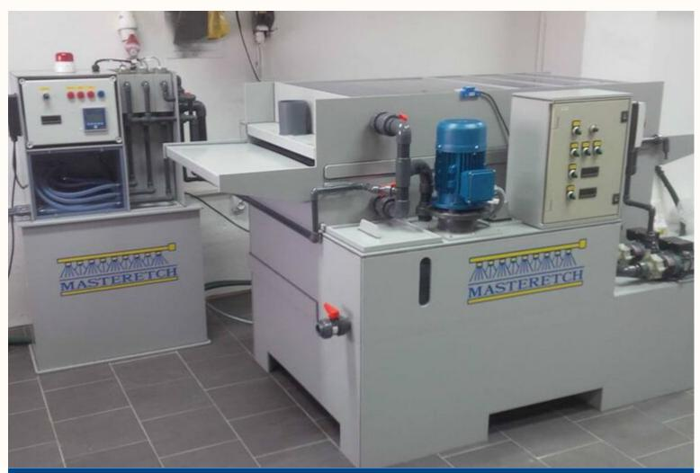
The Model 650 is a powerhouse etching machine ideal for high volume etching and chemical milling operations. The 650 is an ideal machine for customers for whom etching is their main business.
