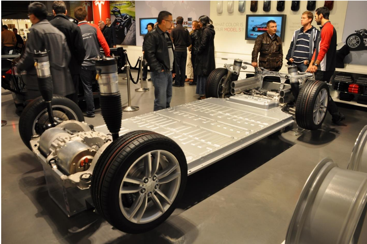
Tesla Model S lithium-ion battery pack in chassis - Photo Credit Marin Gillet via Flickr
