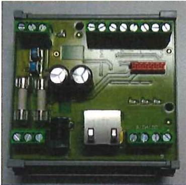
**FLIR ITS 10-6075 R05 Interface: Ethernet connection Box**
