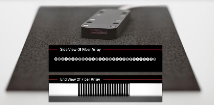
A fiber array for beam-combining applications with 30 PM-LMA fibers. The pictures show 30 LMA fibers with a core/clad diameter of 25/250µm. The fibers are welded to an optical window (16mm x 4.2mm).
