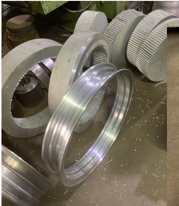
How they started as blocks of billet alloy
