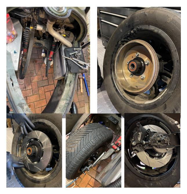
One of the more surprising benefits of fitting this kit, in addition to the improvements in both performance and maintenance, is the fact that the replacement disc components are actually *lighter* than the drum assembly originally fitted. Although the weight savings are not huge, every little helps as they say, not forgetting that this is also unsprung weight and therefore beneficial in terms of suspension load, response and compliance. Here are the figures;
