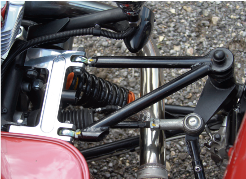
Figure 9 Empire kit adjustable top wishbone. Also shows a ATR shock absorber. (Photo by Simon Goldsworthy)
