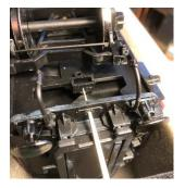
6. Insert MagClic coupling through slot and fix using the supplied spring and split pin as normal. Ensure free movement.
