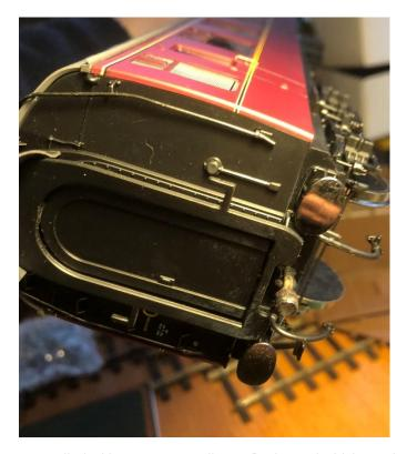
Note: Brake Coaches are supplied with a screw coupling at Brake end which can be changed as per normal if desired.
