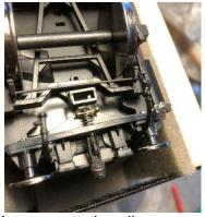
7. Re -affix bogie using screw and spring removed earlier.
