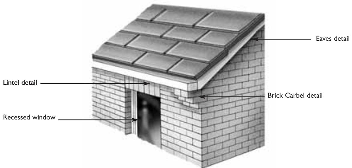
FIG 7. DETAILS The extension should pick up the detail of the main house.
