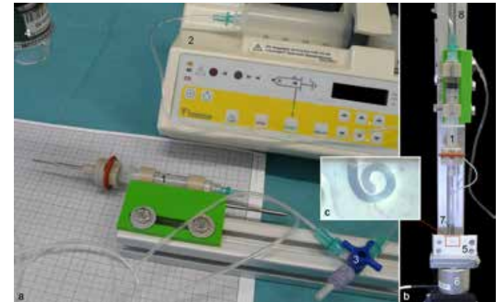
Fig. 2 a Test bench for testing the hydraulic actuation of the probe holder at different velocities. CHD (1) connected to the infusion pump (2). A 3-way Stopcock valve (3) serves to vent the tubing and as an emergency stop. Microscope camera (4) to capture the movement of the probe holder. b Test bench for insertion force measurement. The aCM (5) is fixed on top of a load cell (6). The CHD enables hydraulic actuation of the EA (7) into the model while being fixed to a stand (8). c Inset showing the aCM geometry
