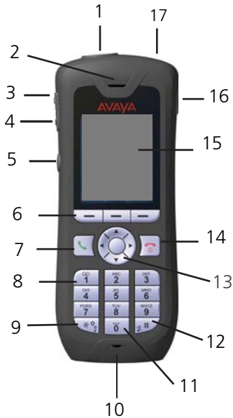
Figure 1: Description of the cordless telephone.
