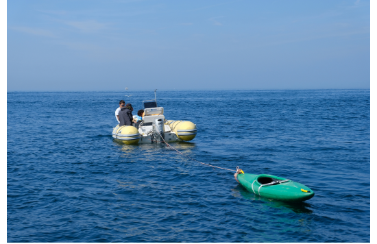
Fig. 2. Boatbot towing a magnetometer
