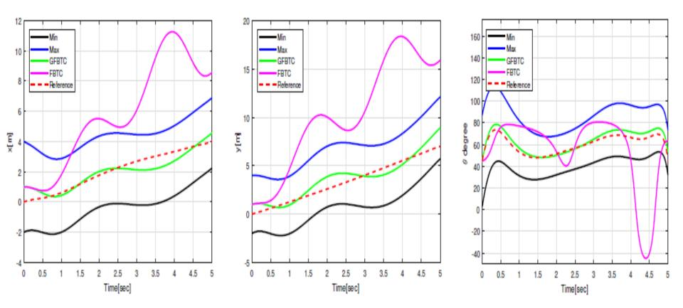
From Simulation 2, the effectiveness of GFBTC can be seen compared to FBTC. Furthermore, the width of the estimated interval increases compared the interval width obtained in simulation 1, and this is due to the augmentation of the value of uncertainties. In spite of this disadvantage, it can be observed that the WMR still moves in a precise interval containing the reference trajectory.
