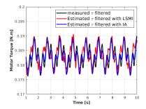
$\hookrightarrow$  The RMSE is around 6.4% with LSMI against 2.6% with IA method, which indicates a reliable fit and a good coherence when the variables uncertainties are accounted.
