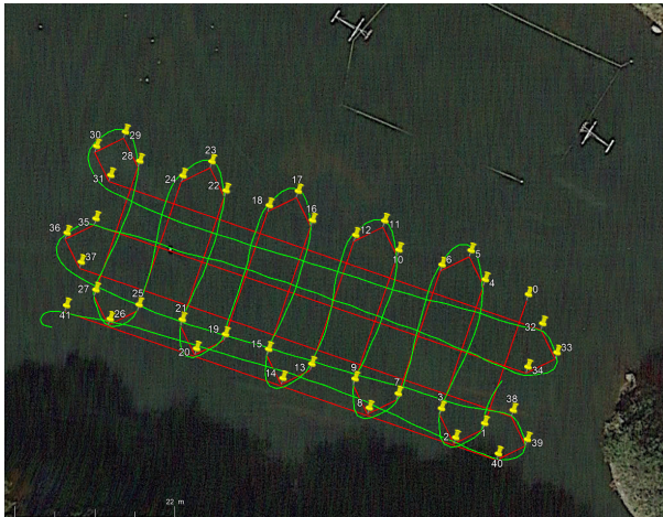
Figure: Real Boustrophedon track (in green) with the desired waypoints (in yellow, connected by red lines). Short legs are approximately 20 m and long ones are 70 m.
