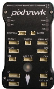
Figure: Example of autopilot typically found on low-cost aerial, surface and submarine drones
