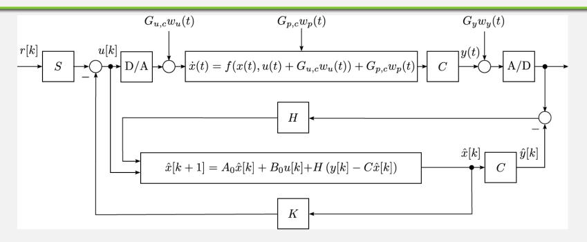
$w_u, w_p, w_y$ : stochastically independent standard normally distributed actuator noise, process noise and sensor noise
