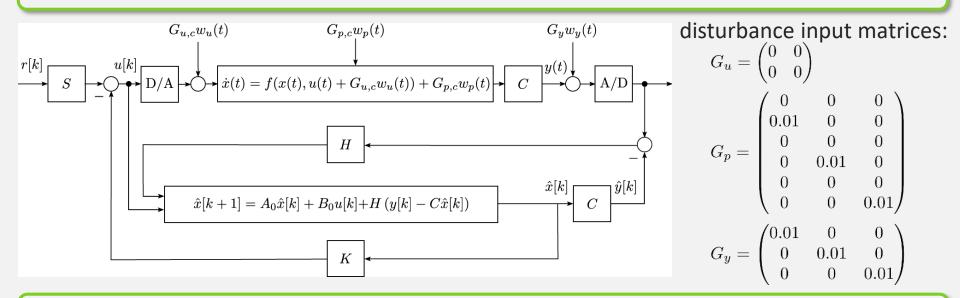
Compared to LQG control: Filter and controller designed separately for the linearized system
