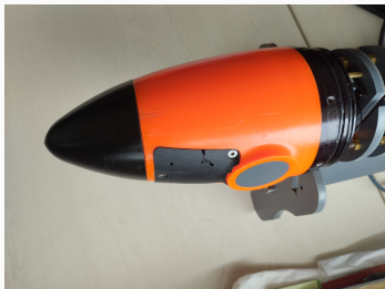
Figure 2: Riptide's echosounder located below the head
