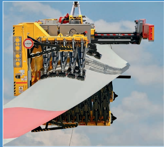
Patent-pending technology: the automatic adaptive blade support of the RBC.
