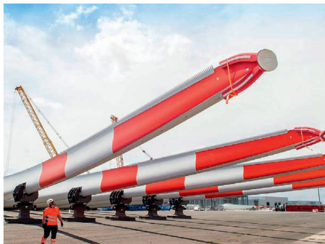
The RecyclableBlade technology is also available for the company's 108m-long B108 blades and the larger 115m-long B115 blades
