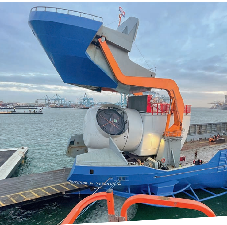
The Rotra Vente has a new overall width of 23.6m, which will enable the transport of seven next-generation nacelles
