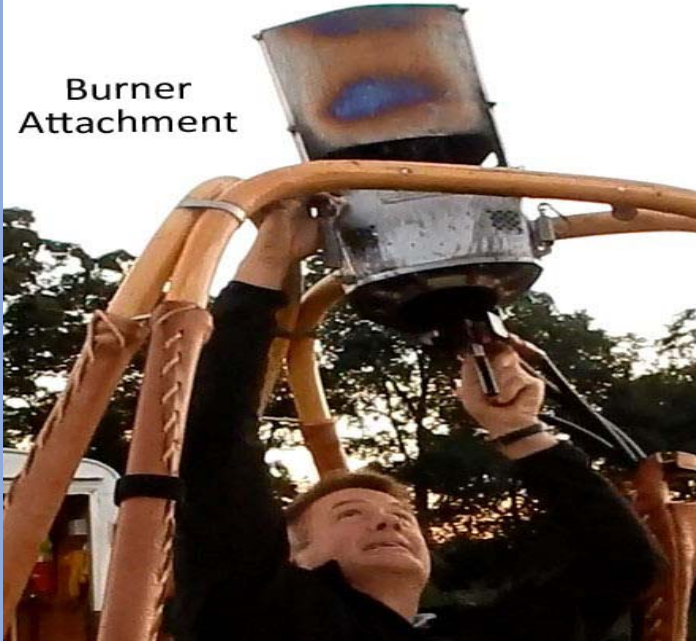
Basket place on side to begin balloon envelope connection inflation
