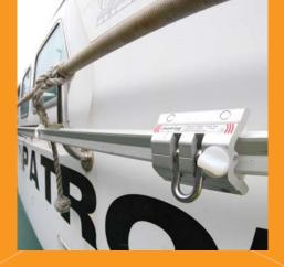
The roller harness carriage or CAR is a revolutionary design of the Hadrian System. The CAR runs on self lubricating delryn wheels which glide easily around the alloy rail. A stainless steel pivoting take off allows lanyard attachment angles between plus or minus 90 degrees whilst maintaining free running of the carriage. The CAR also exceeds the safety specifications of EN795 Class D by a factor of two.
